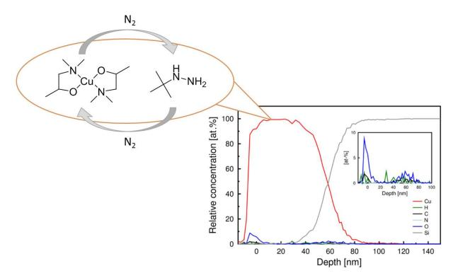
Figure 1. ToF-ERDA results of ALD Cu deposited from Cu(dmap)<sub>2</sub> and TBH at 120 °C.
