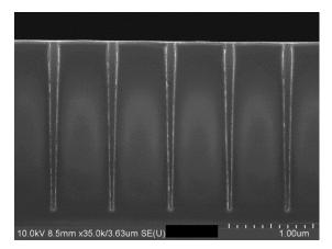
Fig. 2. SEM cross-sectional view of conformal coating of vias by  $O_2$ -free ALD Ru at 225°C
