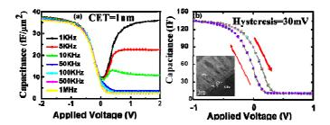
Fig. 1 (a) C-V characteristics of capacitors fabricated using  $Pt/Y_2O_3$  gate stack process on p-Ge. (b) Flat band hysteresis is measured to be less than 30mV.
