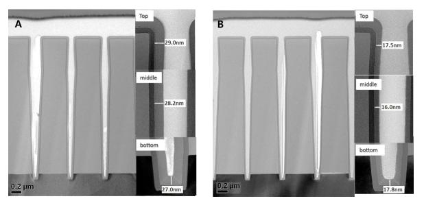
Figure 3. TEM images of a silicon nitride layer on the trench structure with high aspect ratio: (A) as-deposition and (B) post diluted HF etch process. (Silicon nitride film was deposited using  $Si_2Cl_6$ .)
