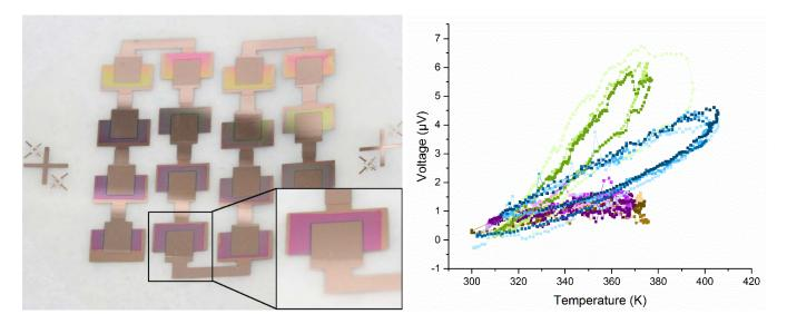
Figure 1: (Left) Photo of the thermoelectric device on the transparent PEN. The thickness of the ZnO layer is around 300nm with some non-uniformity due to the masking tape present during the deposition. On the bottom-right corner a zoomed picture of a single pad is shown.
