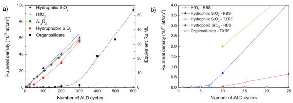
Figure 1: a) Ru coverage measured by Rutherford Backscattering Spectrometry (RBS) for increasing ALD cycle number on -OH terminated hydrophilic SiO<sub>2</sub>, HfO<sub>2</sub>, Al<sub>2</sub>O<sub>3</sub>, Si-O-Si terminated hydrophobic SiO<sub>2</sub>, and Si-CH<sub>3</sub> organosilicate glass, b) inset for low ALD cycle number, showing Ru RBS and Total X-Ray Fluorescence Spectrometry (TXRF) for the initial ALD cycles. Closed lines are provided as a guide to the eye.
