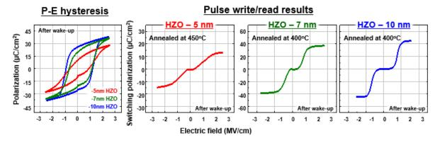
**Figure 2.** P-E hysteresis and Pulse Read/Write measurements of 5nm HZO (annealed at 450°C), 7nm HZO, 10nm HZO (annealed at 400°C). The pulse read/write measurements replicate actual device operation as an FRAM.
