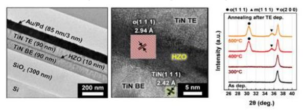
**Figure 3.** The left images show cross-sectional TEM image of the ferroelectric capacitors fabricated using 10nm HZO, annealed at 400°C. The right image shows GIXRD patterns of 10-nm HZO annealed at various temperatures. The figures show that annealing at 400°C is sufficient for proper crystallization of the ferroelectric orthorhombic phase [3].
