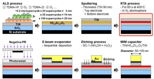
Figure 1. Schematic illustration of the procedure used to fabricate the HZO-based MIM capacitor.
