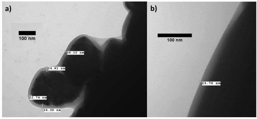
Figure 1. a) 60 cycles of polyamide MLD on  $ZrO_2$  nanoparticles at 67 °C. b) 60 cycles of polyamide MLD on large cellulose particles with diameters of ~200  $\mu$ m at 67 °C. Thickness of polyamide film is in agreement with a MLD growth rate of 4 Å/cycle and consistent on varying sizes and compositions of particles.
