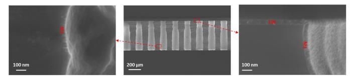
Figure 2. Scanning electron micrographs of TiN coating inside TSVs.
