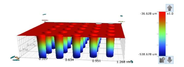
Figure 1. Optical profilometer scan of etched TSVs.
