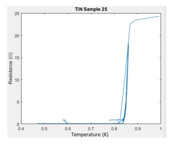
Figure 3. Resistance of an ensemble of TiN coated TSVs as a function of temperature.
