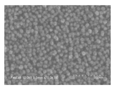
Figure 1. Scanning electron image of the reduced NiO thin-film. Reduction is performed using molecular hydrogen balanced with argon at  $400^{\circ C}$ .
