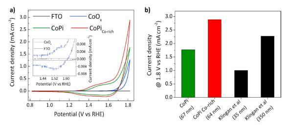
a)Cyclic voltammetry of cobalt oxide, CoPi and Co-rich CoPi thin films after 200 scans at 10 mV/s in KPi buffer 0.1 M (ph= 8) after iR correction. Inset: detail of the oxidative/reductive wave for cobalt oxide and FTO, taken as references. b) Comparison of the current density values of ALD CoPi and Co-rich CoPi at 1.8 V vs. RHE with electro-deposited CoPi [Klingan *et al.*].
