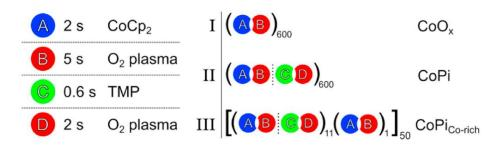
Scheme of the dosing times adopted for the ALD processes of cobalt oxide, CoPi and Co-rich CoPi. Each step of the process is self-limiting and the dosing times are in the saturation region.
