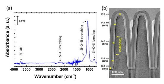
**Figure 2**. (a) In FTIR spectrum, two distinct peaks corresponding to Si–O bonds are observed without any distinguishable Si–H bonds. This implies almost complete transformation of Si–H bonds in TADS to Si–O bonds during the process. (b) The conformality of the PEALD SiO<sub>2</sub> films is shown in high aspect ratio nanotrenches. Based on the high step coverage (>75%), TADS can be potentially used for depositing highly conformal SiO<sub>2</sub> films for semiconductor devices.
