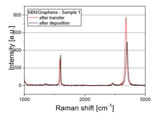
**Figure 1:** Raman spectra displaying Raman band structure for pristine graphene (red line) and post deposition 10 nm of  $Al_2O_3$  (black line). As shown, there is no evidence for damage/defects to graphene as suggested by a D peak intensity below noise level. The ratio between the bands at ca. 2700 and 1600 cm<sup>-1</sup> also suggest high quality graphene has been maintained post-deposition of alumina.
