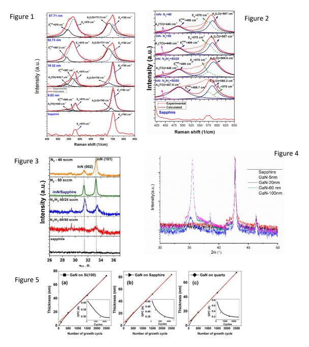
Figure 1 Evalution of Raman spectra for GaN films on Sapphire with different thickness
