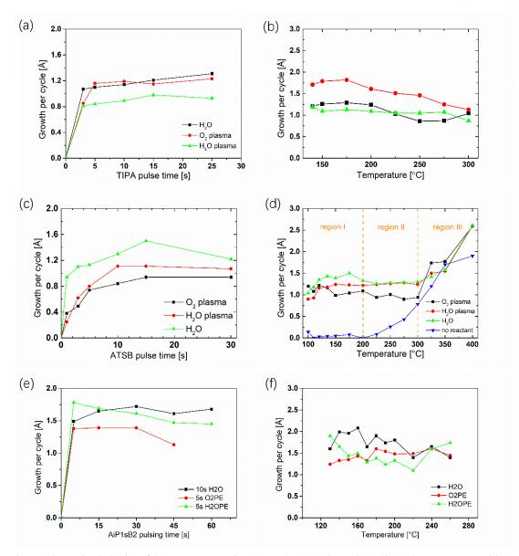
Figure 1 Saturation behavior of ALD processes using (a) TIPA, (c) ATSB and (e) AiP1sB2 as precursors with 5s co-reactants and temperature windows achieved by (b) TIPA, (d) ATSB and (f) AiP1sB2 as precursors.
