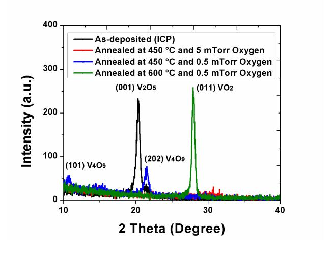
**Figure 1:** Grazing-incidence XRD spectra of PEALD-grown VO<sub>x</sub> thin films: as-grown and annealed under different oxygen pressure and substrate temperatures.
