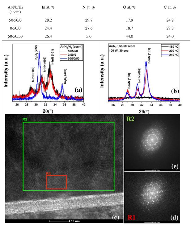
**Table I:** Chemical composition of the 300-cycle InN samples as a function of varying plasma chemistry in terms of atomic concentration (measured from the surface of the films).
