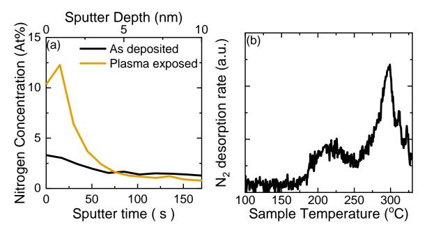
Figure 2: a.) Nitrogen distribution inside an ALD Co thin film exposed to  $NH_3$  plasma as determined by X-ray photoelectron spectroscopy depth profiling. b.)  $N_2$  temperature programmed desorption spectrum of a Co thin film after plasma exposure
