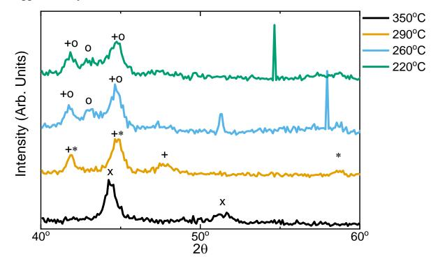
Figure 1: Effect of deposition temperature on the crystal structure of ALD Co and  $CoN_x$  thin films, as determined by grazing incidence x-ray diffraction using Cu K $\alpha$  radiation. Peaks indicated with x and + can be assigned to the FCC and HCP phase of Co respectively, while peaks indicated with \* and o can be assigned to Co<sub>3</sub>N and Co<sub>2</sub>N respectively.
