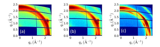
FIG 1. *Ex situ* GIWAXS pattern for  $In_{.62}AI_{.38}N$  superlattices in which each ALEp supercycle consisted of (a) 2/21 (b) 3/30 (c) and 9/90 AIN/INN subcycles. The degree of texturing increases with the superlattice period.
