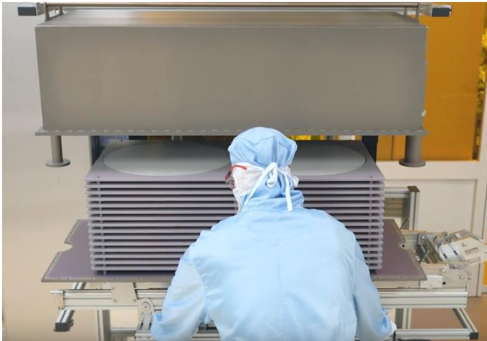
Batch setup used in this study consisted of 30 pcs of showerhead parts (diameter 460mm, thickness 10mm).
