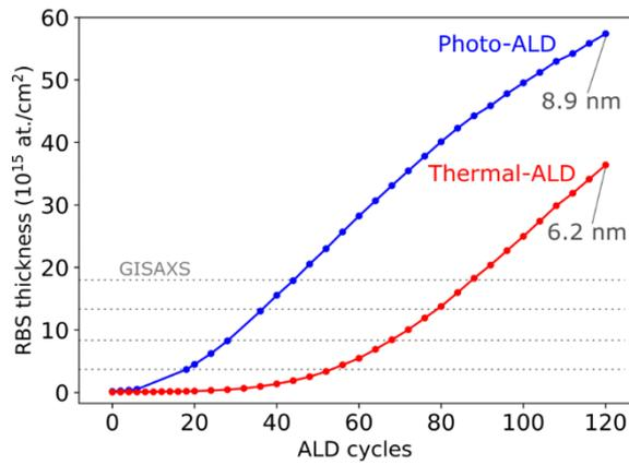
**Fig 1** RBS-calibrated in situ XRF growth curves for Photo-ALD vs. thermal ALD of Pt at 200°C on O<sub>3</sub>-cleaned SiO<sub>2</sub> substrates. The ex situ XRR thickness values measured after 120 ALD cycles are indicated. The horizontal dotted lines represent the Pt loading for which GISAXS data are presented in Figure 3.
