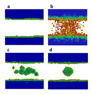
shows formation of a single Si ND via (a)(b) ion beam mixing and (c)(d)thermal treatment.
