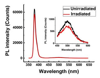
Figure 1: Room temperature photoluminescence spectra of unirradiated and irradiated samples. The inset shows the visible PL spectra.
