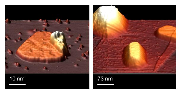
Fig. 1. An intercalated Dy raft with moiré (left) and intercalated Cu islands at 800 K (right). Note that scale bars are different.
