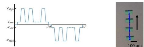
Fig. 1 (left) Waveform primitive applied to the power delivery substrate for actuation.  $V_{low}$  and  $V_{high}$  represents the lowest and highest voltage level respectively of pulse train (250 pulses) shown for one cycle. (right) Composite optical micrograph showing representative USDA motion on power delivery substrate. Motion is recorded for  $V_{low}=0V$  and  $V_{high}=170V$  at 15Hz frequency for deposition pressure of 25 mTorr. Position of USDA is recorded every 250 frames.
