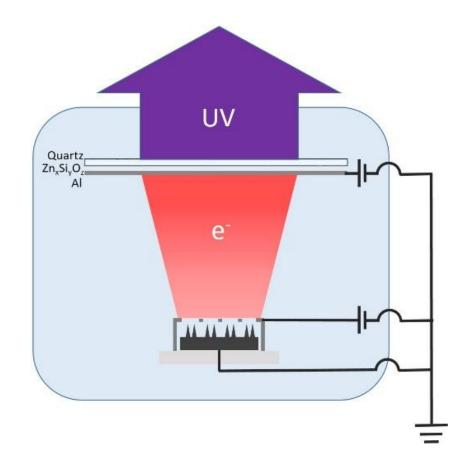
Schematic of UV light generation with CNT based cold cathode electron beam. For electron irradiation C-beam structure optimized
