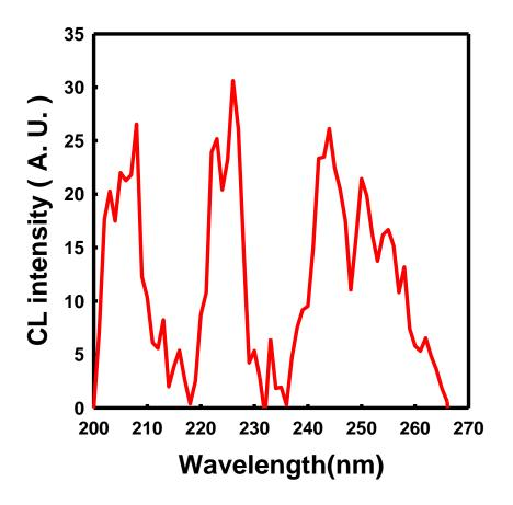
Emission peak of UV light with CNT based cold cathode electron beam. Peak position depend on the anode layer fabrication process.
