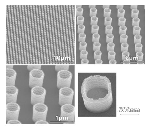
Figure 1. SEM micrographs revealing the metallic-glass nanotube array at different magnifications.
