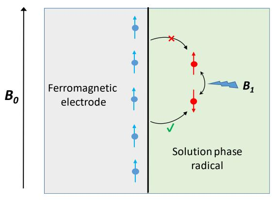
Figure 1: An electrochemical interface between a ferromagnetic electrode and a solution. The electrons from the electrode are transferred to the radical species in the solution preferentially when the spins of the electrons are antiparallel.
