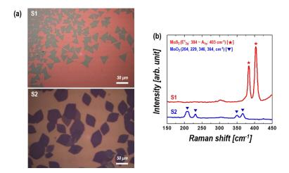
Figure. 1 (a-b) Optical image and Raman spectra of  $MoS_2$  and  $MoO_2$  crystals by CVD
