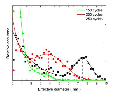
Figure 2: Size distribution of ALD cobalt nanoparticles as a function of the number of deposition cycles. Lines as a guide to the eye
