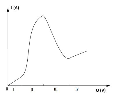
Figure 1. Current-voltage relationship for the process of cathodic plasma discharging.
