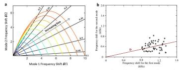
Figure 3. (a) Two-mode frequency shift domain. The straight contour lines are for position (normalized to unity, so 0.5 means the center of the beam). The contours for mass are shown as circular-shaped curves. (b) Initial location measurement in this study, representing the passage of a single cell from capillary D (in  $1/3^{rd}$  of resonator length).
