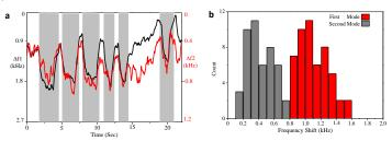
Figure 2. (a) Two-mode frequency shifts due to Skbr3 wt breast cancer cell passage measured by two parallel PLLs; the black trace shows the first mode, and the red trace shows the second mode. The offset frequencies of fl = 974.734 MHz and f2 = 1.85774 GHz are subtracted for clarity. (b) Histogram of the frequency shift amount in both modes.
