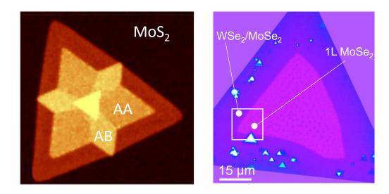
**Figure 1:** 2D homo-(left) and hetero-junction grown by CVD method.
