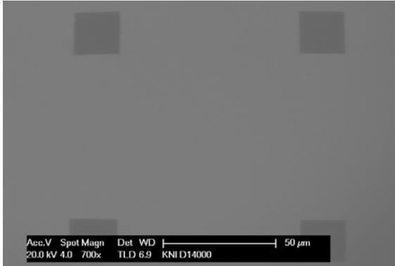
Figure 4. SEM micrograph in immersion mode of 20 micron squares fabricated directly in resist for use as alignment marks
