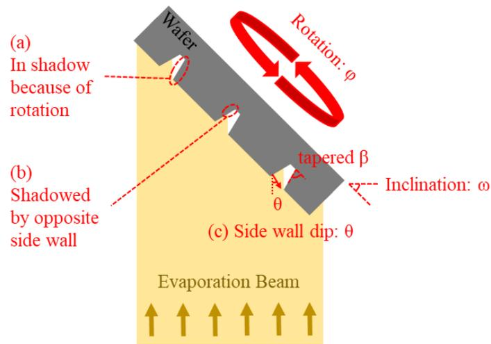
**Figure 1: Schematic diagram of inclined electron beam evaporation**
