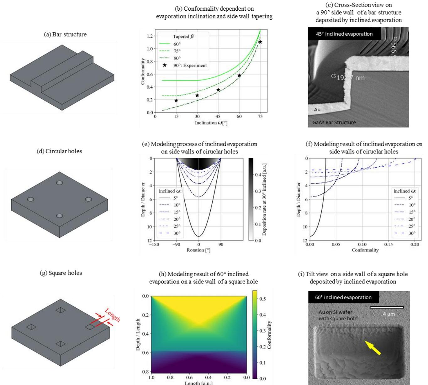
**Figure 2: Physical model and experimental results of inclined evaporation on side walls**
