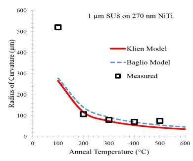
Figure 2 measured and modeled curvature radius for SU8 on NiTi devices vs. SU8 cure temperature
