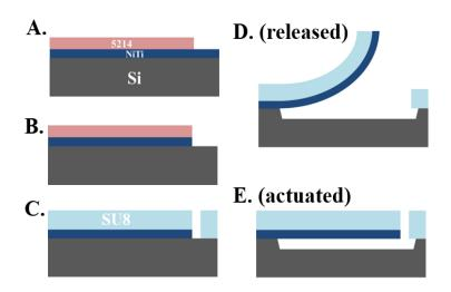
Figure 1 microfabrication process for SU8 on NiTi devices
