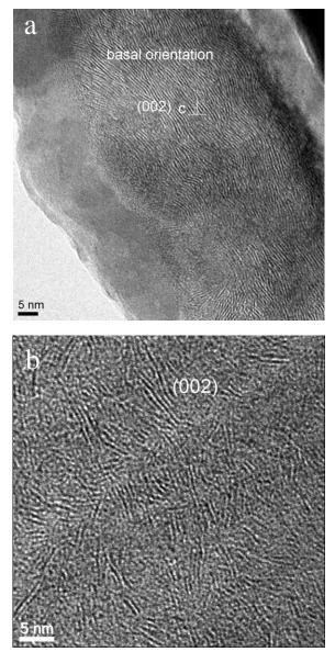
Fig.1. TEM images: a) Pure  $WS_2$  showing clear basal orientation; b)  $WS_2$ /a-C coating showing  $WS_2$  platelets randomly distributed in amorphous carbon matrix.
