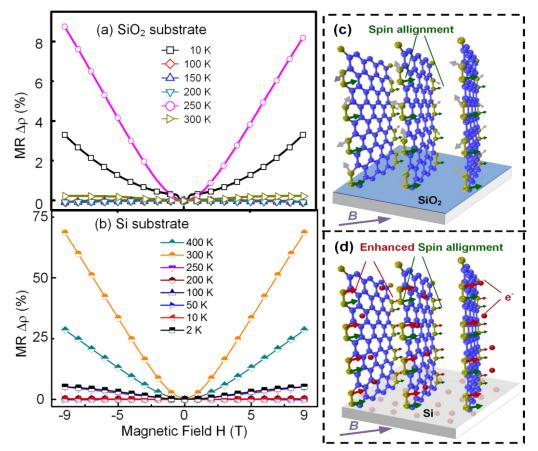
Fig. 1. MR performances of nanocrystallited carbon films on (a) Si and (b) SiO<sub>2</sub> substrate. The spin alignment mechanism is illustrated in figure (c) and (d)
