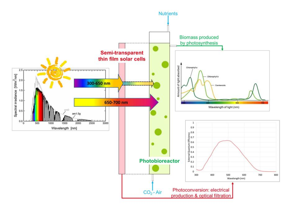
Figure 1: a PBR/Semi-transparent thin film solar cell coupled system
