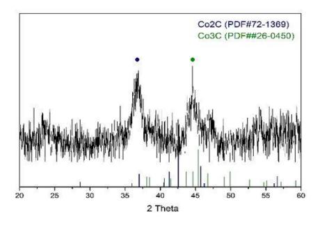
XRD of Co<sub>3</sub>C and Co<sub>2</sub>C with TEG and NaOH and react at 300°C for 2 hr.
