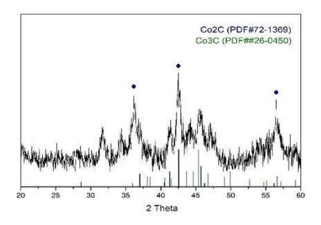
XRD of Co<sub>2</sub>C with TEG and OLA react at 300°C for 3 hr.
