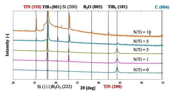
Figure 2 XRD results of as-deposited TiBN thin films with different N/Ti ratio.
