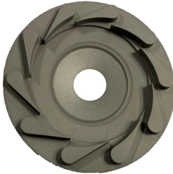
Figure 1. Refractory-element thermal coating using atmospheric plasma spray (APS).
