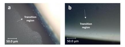
Fig. 1: Representative Nomarski images of the grown layers on a) (111)B and b) (111)A substrates at optimum growth conditions taken at the wafer edge.
