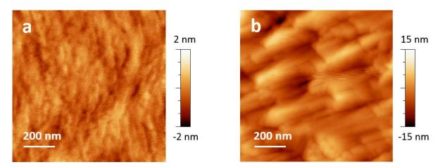
Fig.S.2: AFM height mode images of the grown epilayers of a) (111)B and b) (111)A. Images are taken at the optimum vicinal surfaces region.
