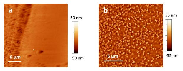
Fig. S.1: AFM height mode images of the grown epilayers on the exact a) (111)B and b) (111)A. The panel (a) shows the transition between the rough and smooth regions.
