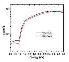
Figure 2. Optical absorption spectra of Zn<sub>3</sub>N<sub>2</sub> films.
