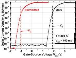
Fig. 1: Normally-off transfer characteristics of an FET fabricated form a GaN/AlGaN heterostructure without a conductive channel at 300 K in the dark. A channel is formed under UV exposure, which results in normally-on FET operation.
