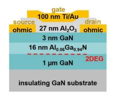
Fig. 4: Cross-sectional illustration of a lateral FET fabricated from a GaN/AlGaN heterostructure with no 2DEG present in the dark. The overlap of gate and source/drain contacts is essential for FET operation, since only underneath the gate electrode a 2DEG can be generated electrostatically. Gate and source/drain contacts are separated by a highly insulating dielectric layer.
