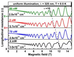
Fig. 2: Low temperature longitudinal magnetoresistance of a Hall bar device under steady UV excitation at different power. An increase in the illumination power of almost 5 orders in magnitude only raises the channel density by 20 %.
