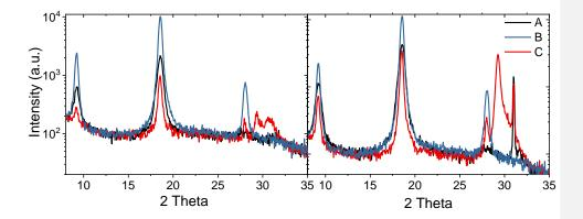
Figure S1: XRD scans of samples A-C with the GaAs substrate oriented A) parallel or B) perpendicular to the XRD beam path. Not the emergence of the (105) peak in sample C and its dependence on substrate orientation.
