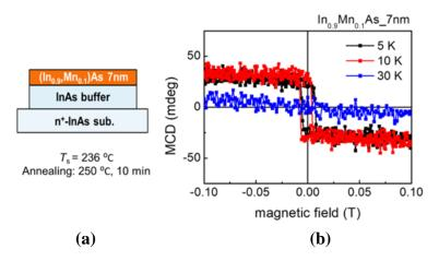
Fig 1. (a) Growth of InMNAs on InAs. (b) Shows pristine quality of the ferromagnetic ordering with Curie temperature below 30K.
