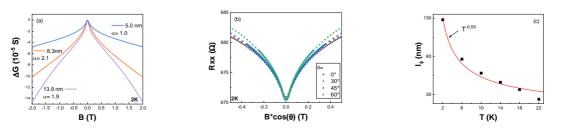
Figure 1: a) Magnetoconductance of samples with different superlattice period thickness. b) Angle dependent magnetoresistance and c) Dephasing length  $(l_{\phi})$  as a function of temperature of the 5 nm period superlattice.
