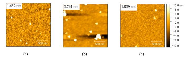
Figure 2:  $2x2\mu m^2$  AFM images of InGaN thin films on Zn-face ZnO substrates with changing Ga flux: (a) 1e-7, (b) 1.5e-7 and (c) 2e-7 Torr showing RMS roughness of 1.652 nm, 3.761 nm and 1.039 nm, respectively. The inset values show the RMS values of the thin films.
