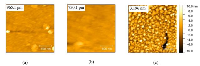
Figure 3:  $2x2\mu m^2$  AFM images of InGaN thin films on O-face ZnO substrates with changing Ga flux: (a) 1e-7, (b) 1.5e-7 and (c) 2e-7 Torr showing RMS roughness of 965.1 pm, 730.1 pm and 3.196 nm, respectively. The inset values show the RMS values of the thin films.
