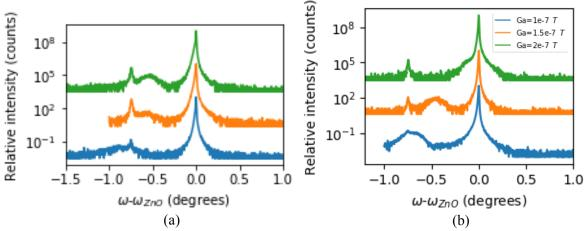
Figure 1: XRD  $2\theta - \omega$  profile along the (002) direction showing InGaN thin films grown on (a) Zn-face (b) O-face ZnO substrates with different Ga fluxes:  $1x10^{-7}$ ,  $1.5x10^{-7}$  and  $2x10^{-7}$  Torr. The Zn-face ZnO substrates show In incorporation 35%, 26%, 21%, respectively. The O-face ZnO substrates show In incorporation 31%, 15%, 6%, respectively.
