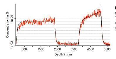
**Figure 2.** Si-doping profile in an InP nanowire as obtained by Atom Probe Tomography. Muraki-type fits where used to describe the quality of the doping interfaces.
